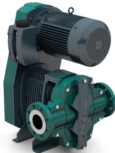
FIGURE 3. Netzsch's Tornado T2 rotary lobe pump features an elastomer housing liner and steel lobes and can be fully serviced through its front cover
