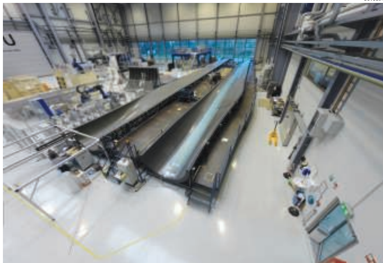
FIGURE 3. Polyurethane-based composites have been used to create large components for wind-turbine blades, including a 45-m spar cap
