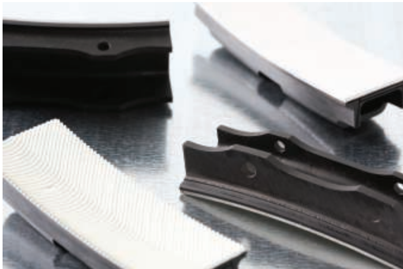
FIGURE 4. High-pressure turbine shrouds constructed of ceramic matrix composites (CMCs) are resistant to the extreme temperatures experienced in jet engines
